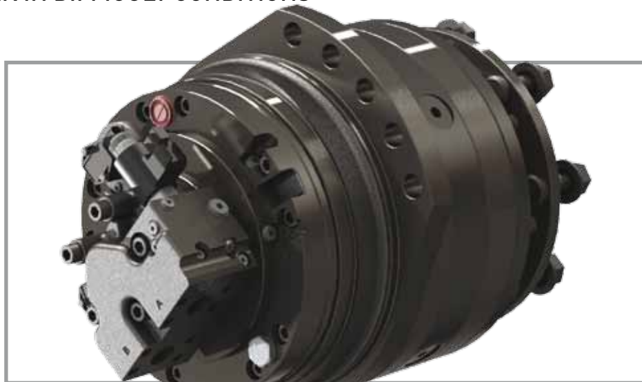
ABOVE: Compact five-piston variable-displacement wheel drive unit with integrated gearbox and brake. Supplied with a complete electronic control package, the sturdy unit also features heavy-duty bearings and high-speed capacity
